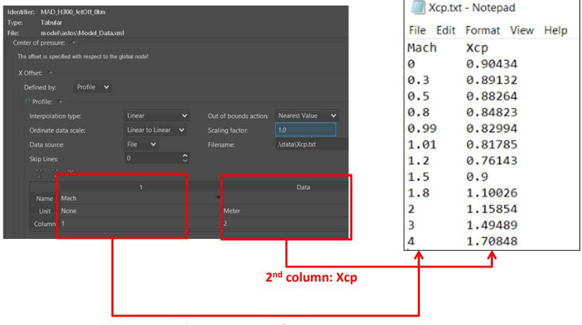
1<sup>st</sup> column : Mach (Values must be monotonically increasing)
