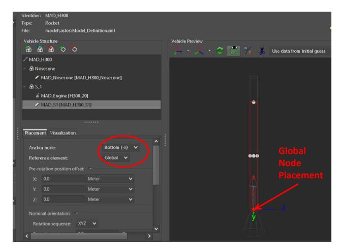
In this case, XCP is defined +ve since global node is at the bottom. In the case where global node is placed at tip of nose, XCP should be defined -ve.
